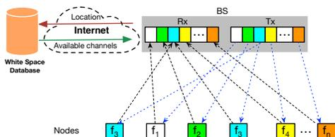
Fig. 1. SNOW with dual radio BS and subcarriers. As shown in Figure 1, the BS uses two radios, both operating on the same spectrum – one for only transmission (called **Tx radio**), and the other for only reception (called **Rx radio**). Such a dual-radio of the BS allows concurrent bi-directional communication in SNOW.
