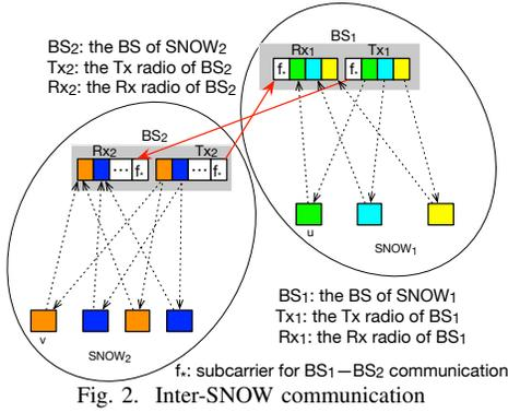
by exploiting the PHY design of SNOW. To explain this we consider *peer-to-peer* (P2P) communication between two SNOWs. That is, one node in a SNOW wants or needs to communicate with a node in another SNOW.
