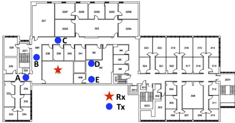
Fig. 9. Node positions on building floor plan.
